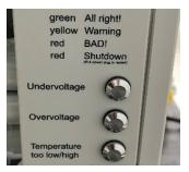
The HY-115 Pump is equipped with three colored LED lights integrated into the electric control box for system monitoring. The LED lights let you know that you are operating within voltage and temperature limits.
