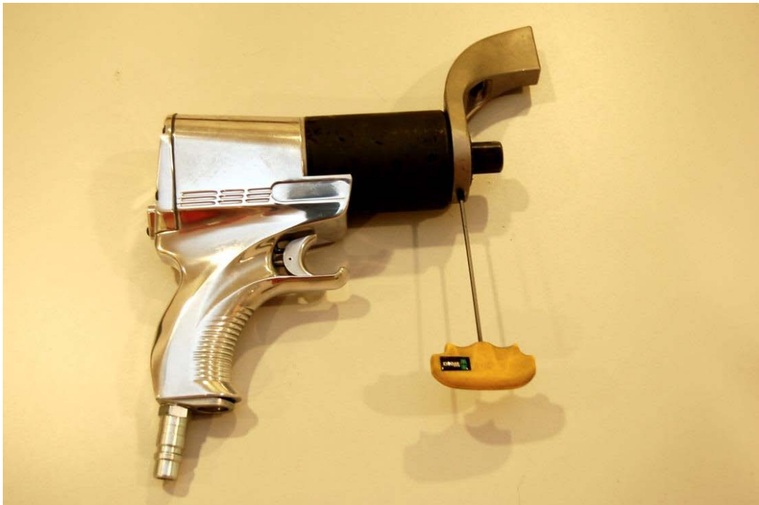
Figure 5. Tightening Reaction Arm Set Screw
