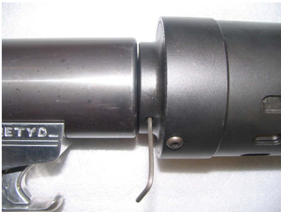
Figure 27. Tightening HYTORC Washer™ Set Screw
