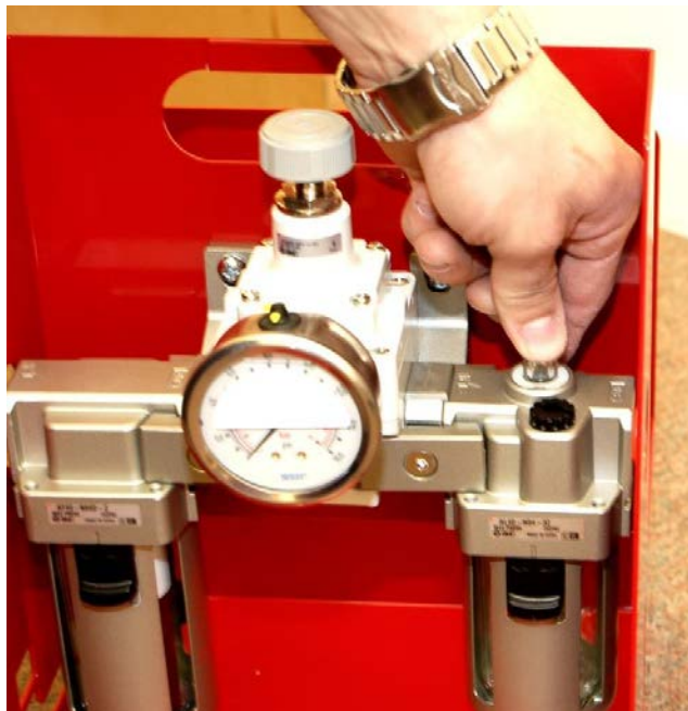
Figure 22. Adjusting FRL Oil Flow
