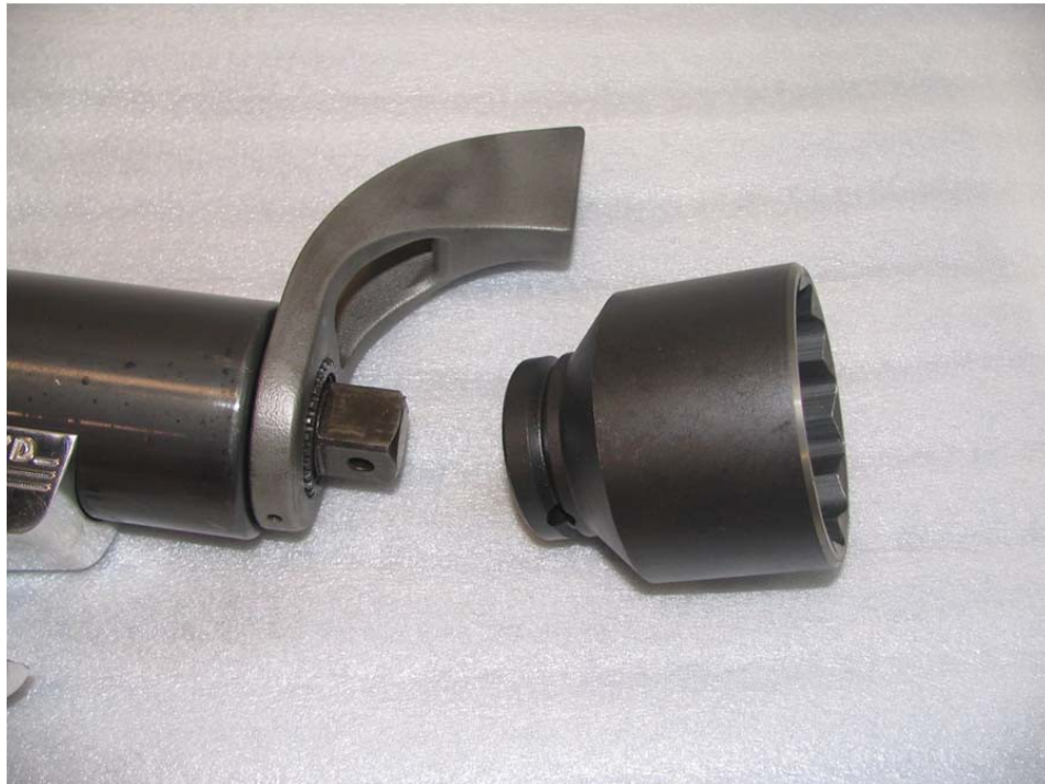
Figure 6. Installing jGun Socket
