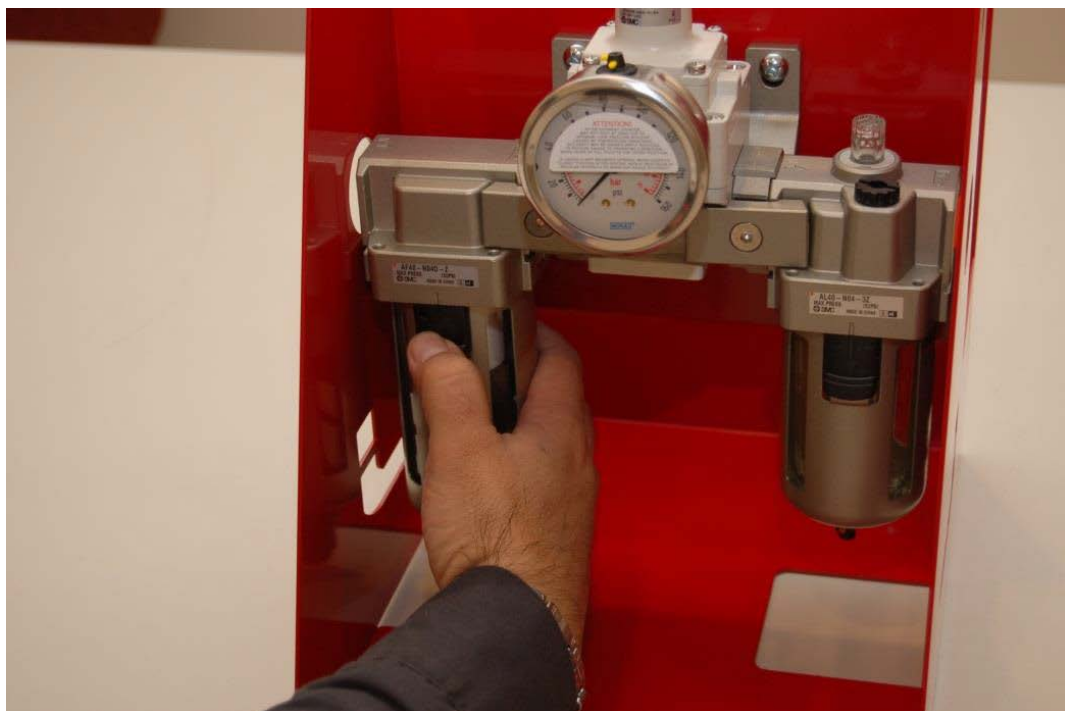
Figure 18. Emptying the FRL Filter Reservoir
