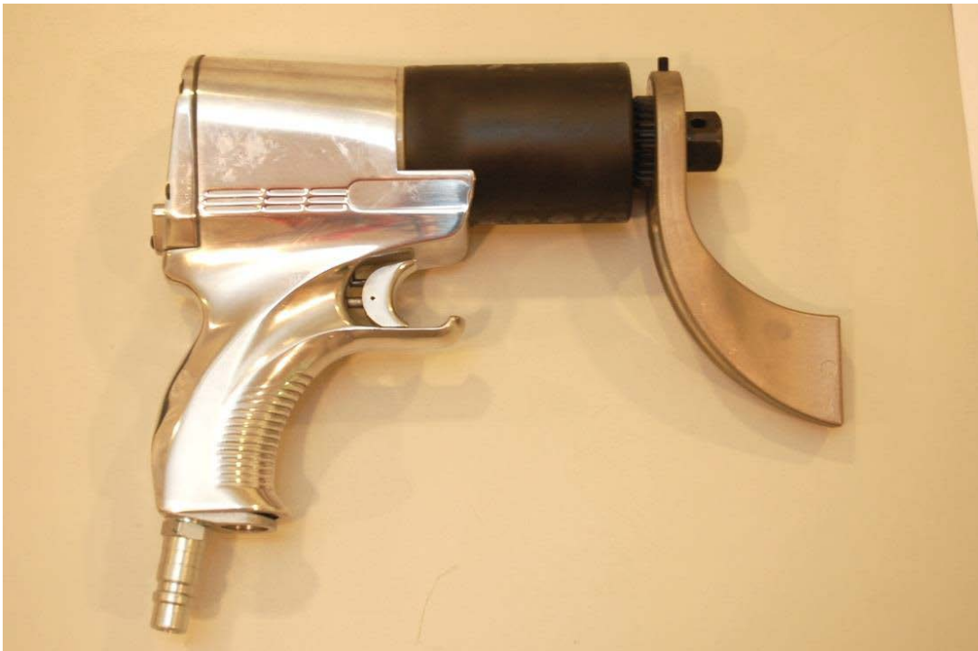
Figure 4. Reaction Arm Installed
