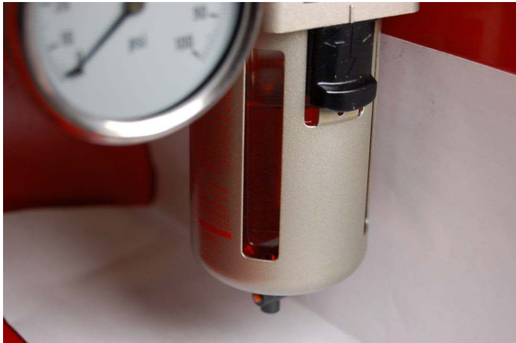
Figure 20. FRL Unit – Lubricator 2/3rds Full of Oil
