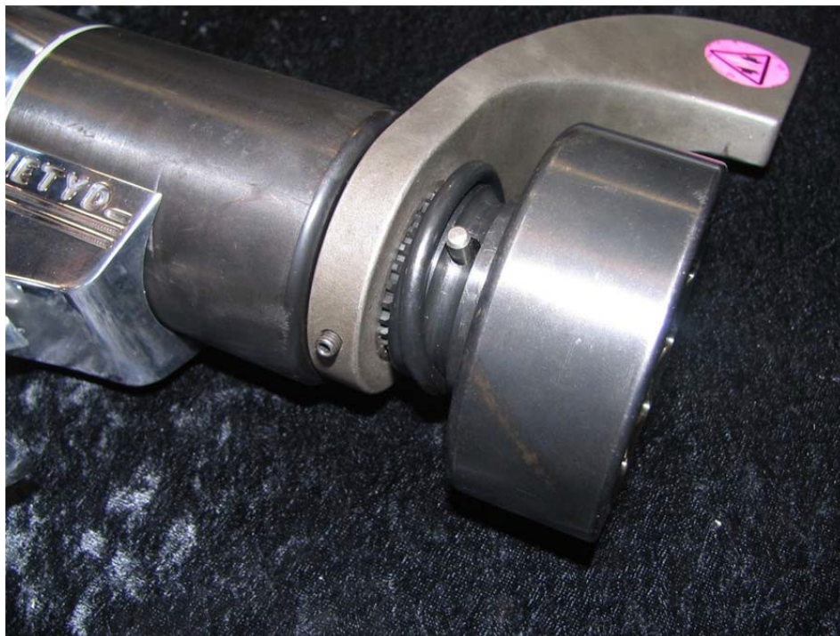
Figure 7. Installing Socket Locking Pin and Retaining Ring
