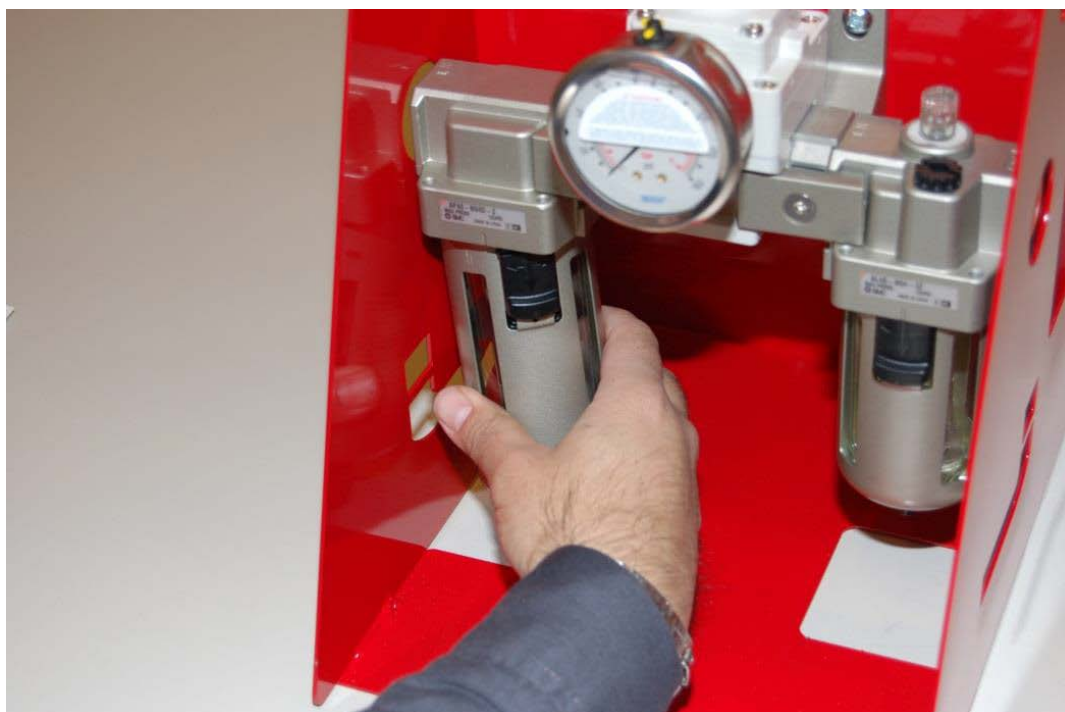
Figure 19. Detaching FRL Reservoir
