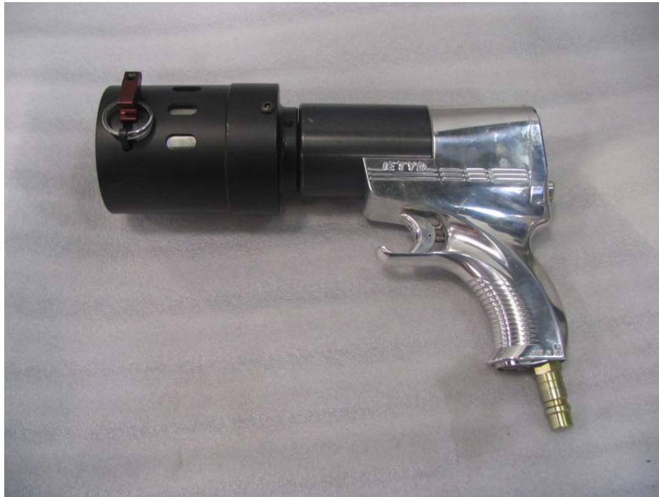
Figure 24. HYTORC Washer Socket Mounted on jGun
