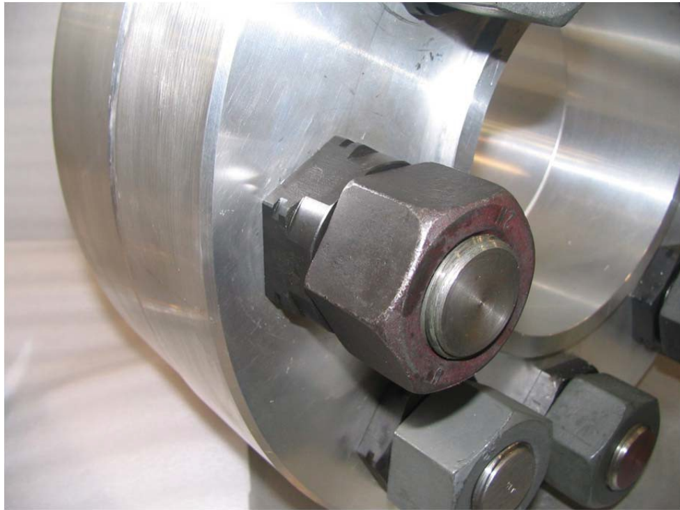
Figure 25. HYTORC Washer Installed
