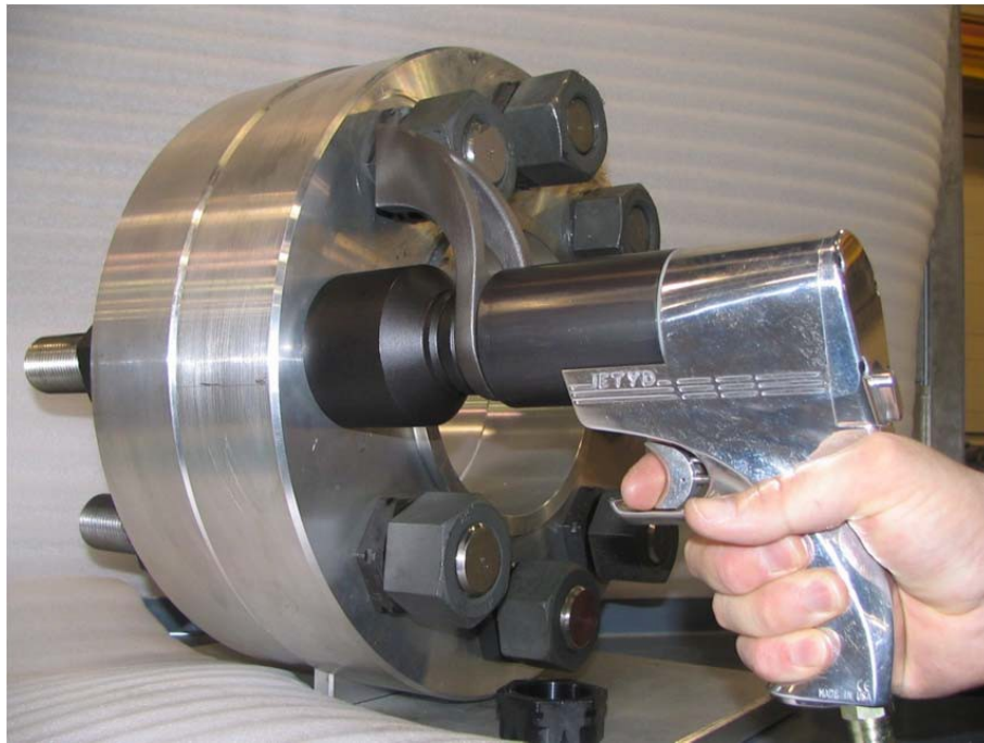
Figure 11. Using the jGun with a Reaction Washer
